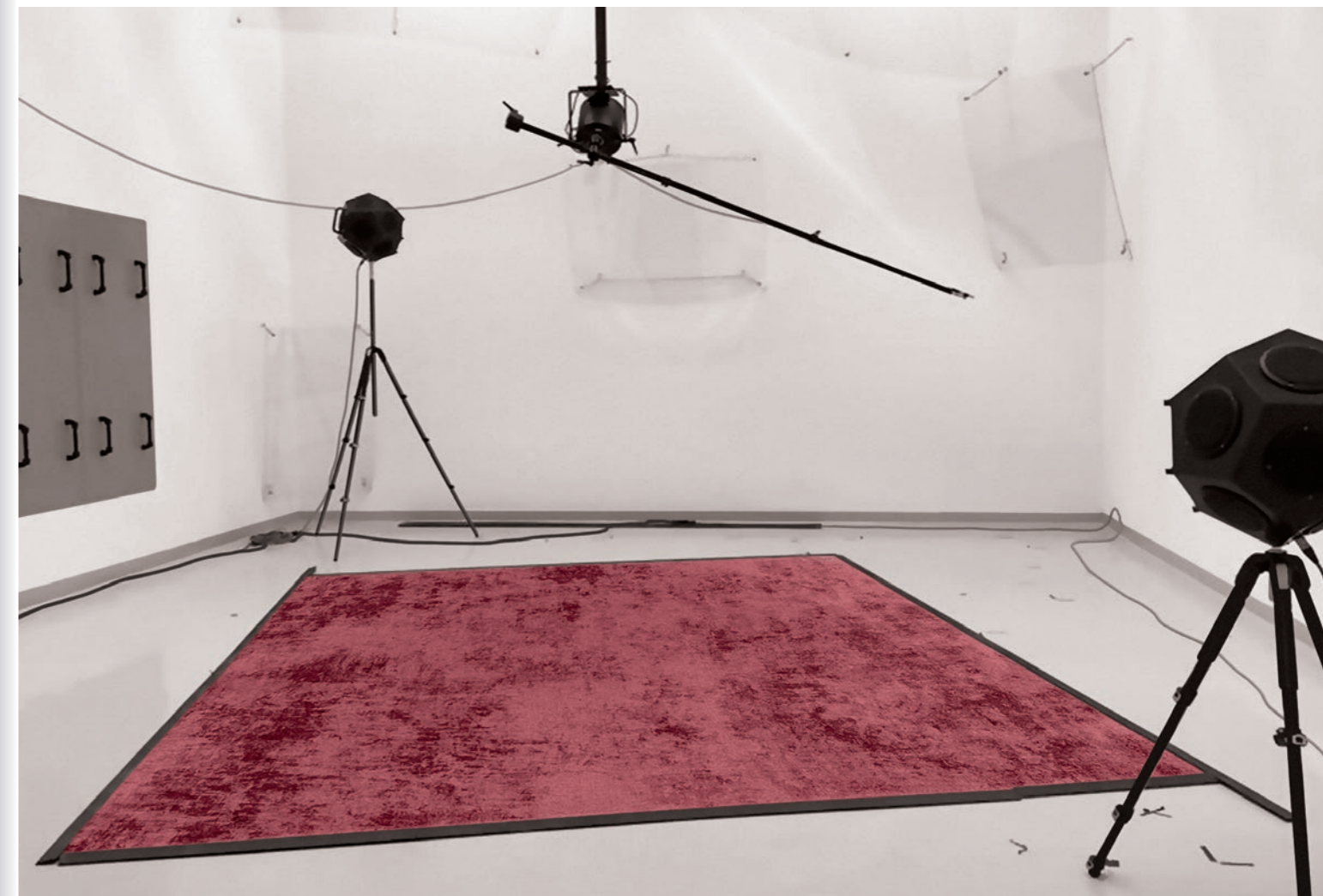
Fig. 61: TFI echo room with loudspeakers, microphone, diffusers and test specimen; source: TFI Aachen
