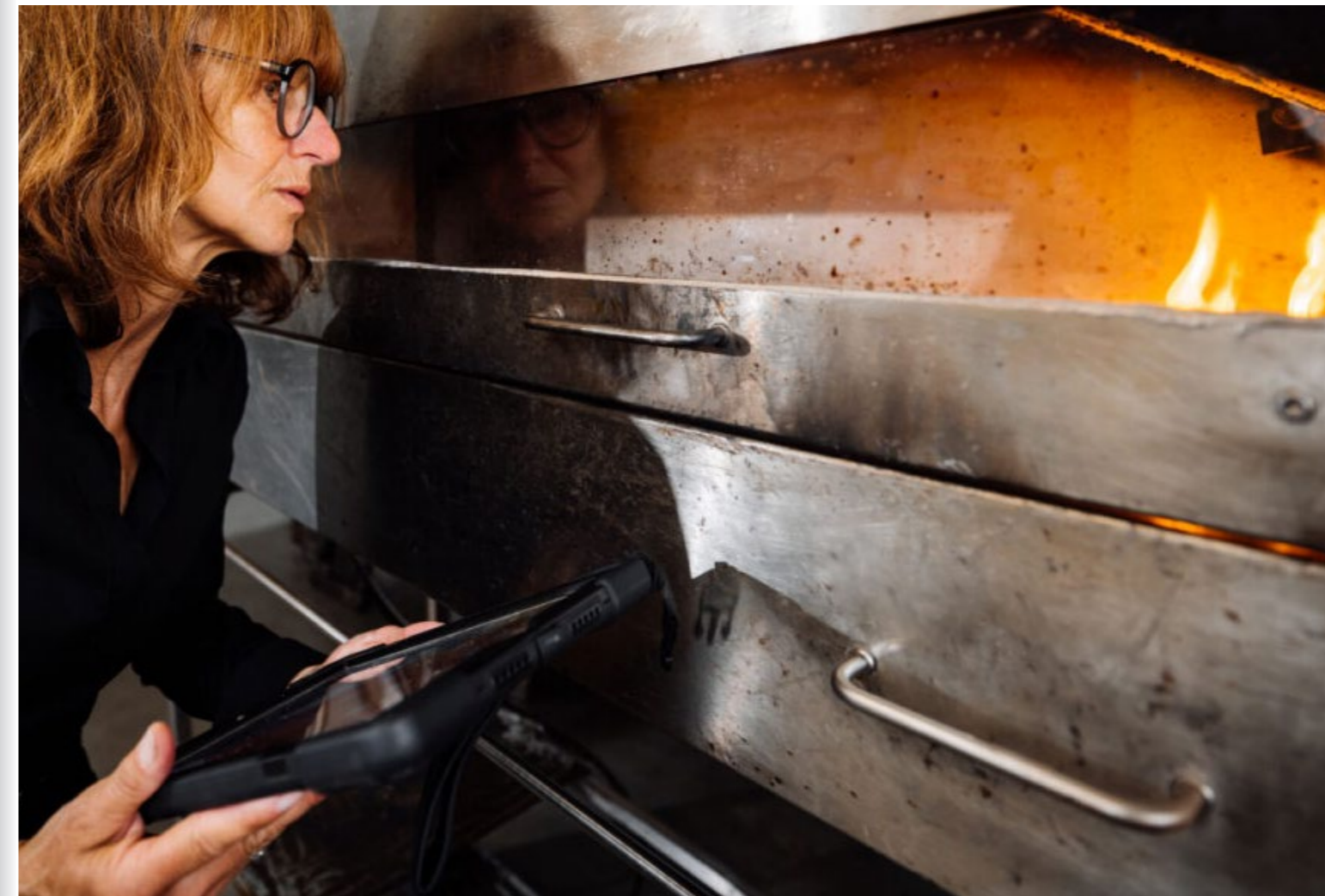
Fig. 65: recording the progress of the fire in the „Radiant Panel“ test chamber; source: TFI Aachen
