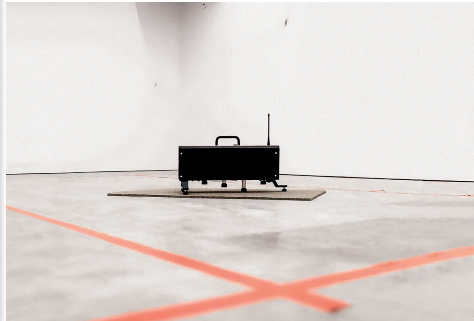
Fig. 59: tapping machine in the upper test room during impact sound reduction test; source: TFI Aachen
