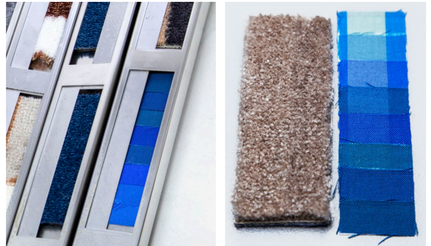
Fig. 40: test specimen and blue scale before exposure Fig. 41: test specimen and blue scale after exposure
